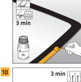
check for contamination ■ If contaminated, scrub the bonding surface with Sika® Cleaner PCA
