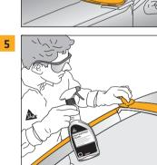
Remove debris with a vacuum cleaner or brush Clean the entire aperture with Sika® Cleaner G+P, making sure the surface
