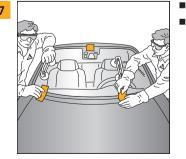
Dry fit the windshield To ensure a quick and precise installation of the windshield once the adhesive is applied, add fitting marks
